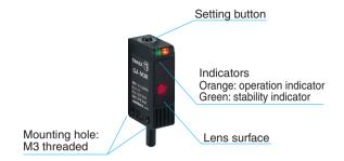
This sensor only has one setting button and no sensitivity adjustment volume or selector switch. Light-ON/Dark-ON switching and sensitivity setting are handled with the setting button alone.
