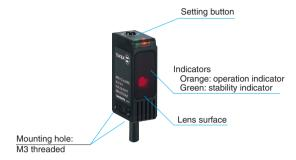
This sensor only has one setting button and no sensitivity adjustment volume or selector switch. Light-ON/Dark-ON switching and sensitivity setting are handled with the setting button alone.
